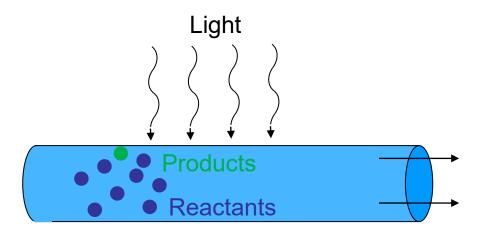
Later on (further down the tube) Lower reaction rate
