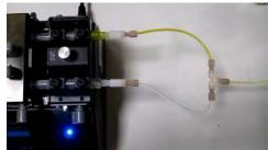
Pumping – dual syringe pump Mixing – tee piece
