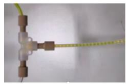
Pipe reactor – segregated droplets of water and oil
