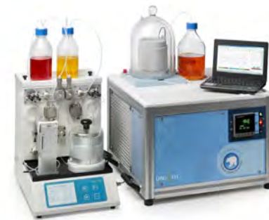
FlowSyn with Polar Bear cryogenic reactor module
