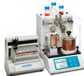
Integrated flow chemistry synthesis system with automated control
